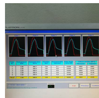
Figure 3. Determination of stiffness modulus on cylindrical samples, IT-CY
