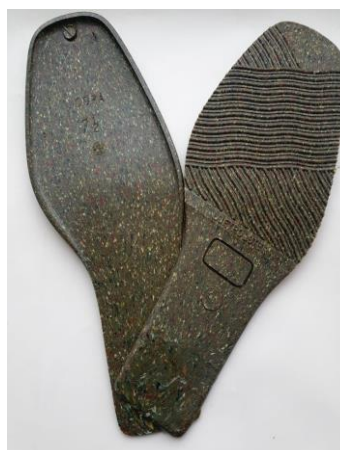
Soles from PVC mixed with 10% ground EVA of 0.5 mm granulation
