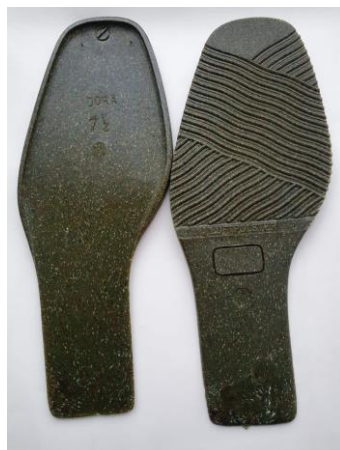
Soles from PVC mixed with 10% ground EVA of 0.35 mm granulation
