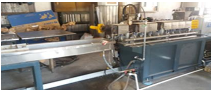
Figure 3. Double screw granulator extruder with corotation TSE 35 type
