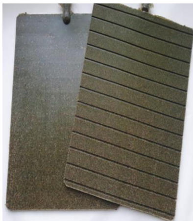
Plate from PVC mixed with 10% ground EVA of 0.35 mm granulation
