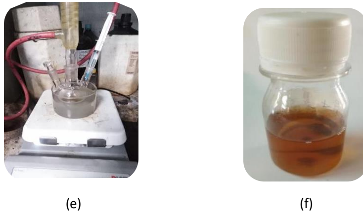
Figure 6. Enhancement of retanning agent derived from tannery waste hair, specifically addressing: (a) Hair waste, (b) Crushed hair, (c) Alkali hydrolysis, (d) Keratin hydrolysate (KH), (e) Graft polymerization process, (f) Developed retanning (KRA)
