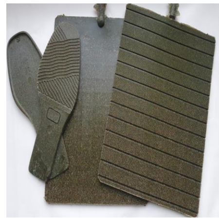
Plate and soles from PVC mixed with 10% ground EVA of 0.35 mm granulation
