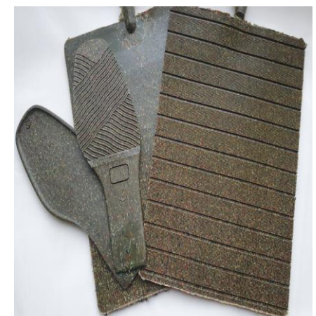
Plate and soles from PVC mixed with 10% ground EVA of 0.5 mm granulation
