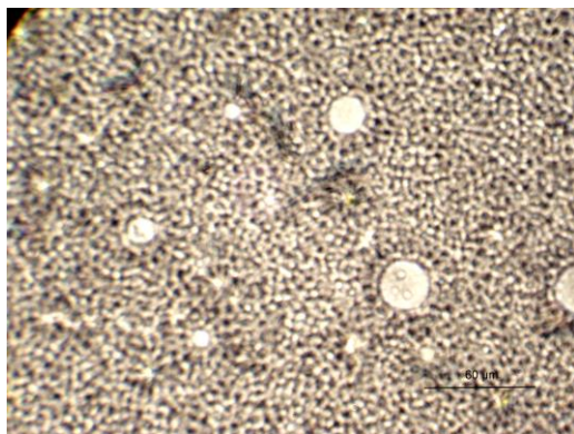
Figure 5. Micrographs of PCL1 adhesive (100 CR: 30 CIIR) in: a) unpolarized light, b) polarized light, after standing of the film for 72 h
