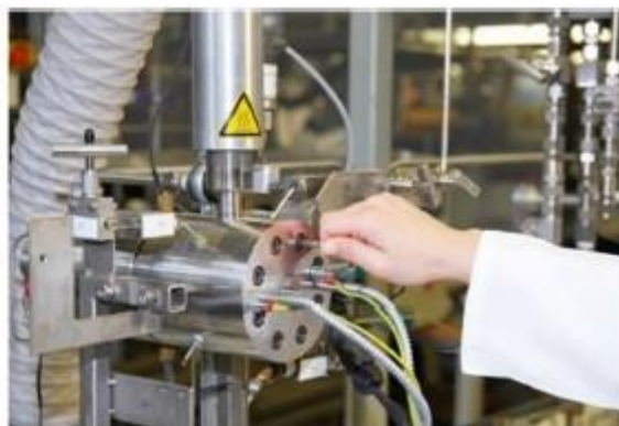
Figure 1. Experimental set-up – high-pressure view-cell for SFE operations
