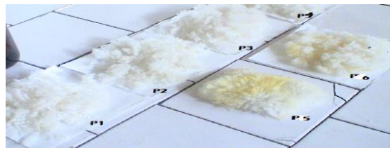
Figure 7. Image of fur samples bioprocessed with enzymes: samples P1-P6
