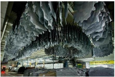
Figure 5: Toggle and crust air drying
