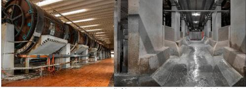
Figure 3: Beamhouse drums (left) and unloading channels (right)
