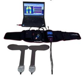
Figure 3. The Pedar-X in-shoe plantar pressure measurement system used for data collection
